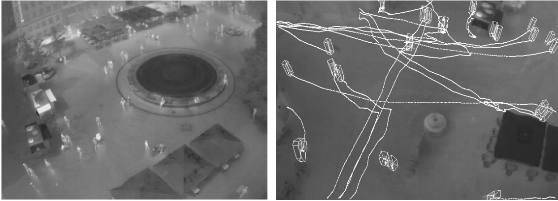
Figure 1. The two scenes recorded by the thermal camera in our pilot study. Tracks captured by manual digitizing in T-Analyst are overlaid on the image to the right.
