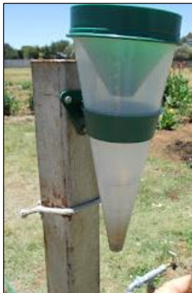
Figure 3. Rain gauge for rainfall measurement
