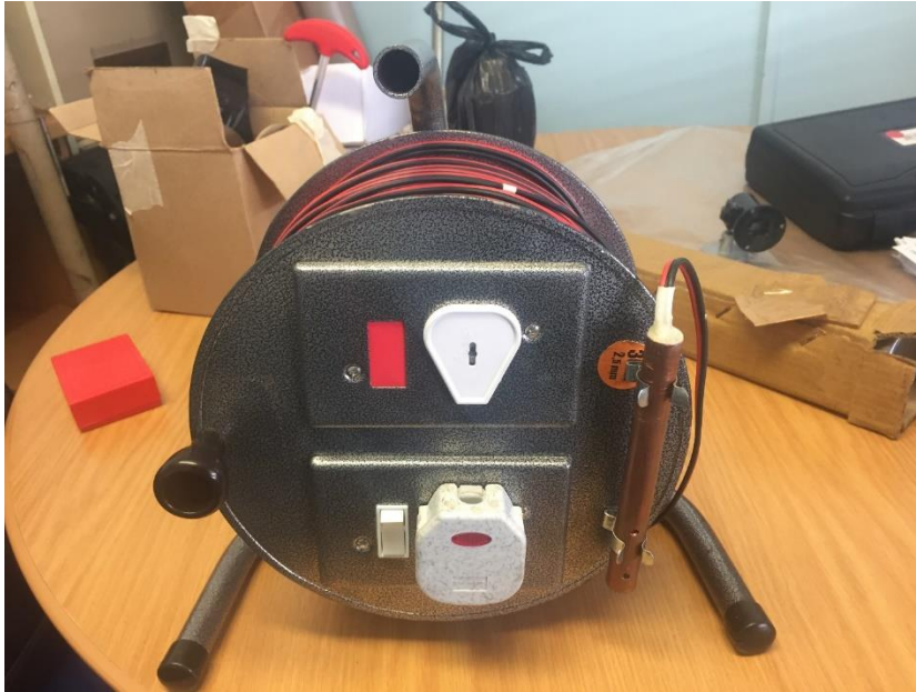
Figure 2. Groundwater level meter for groundwater level measurement
