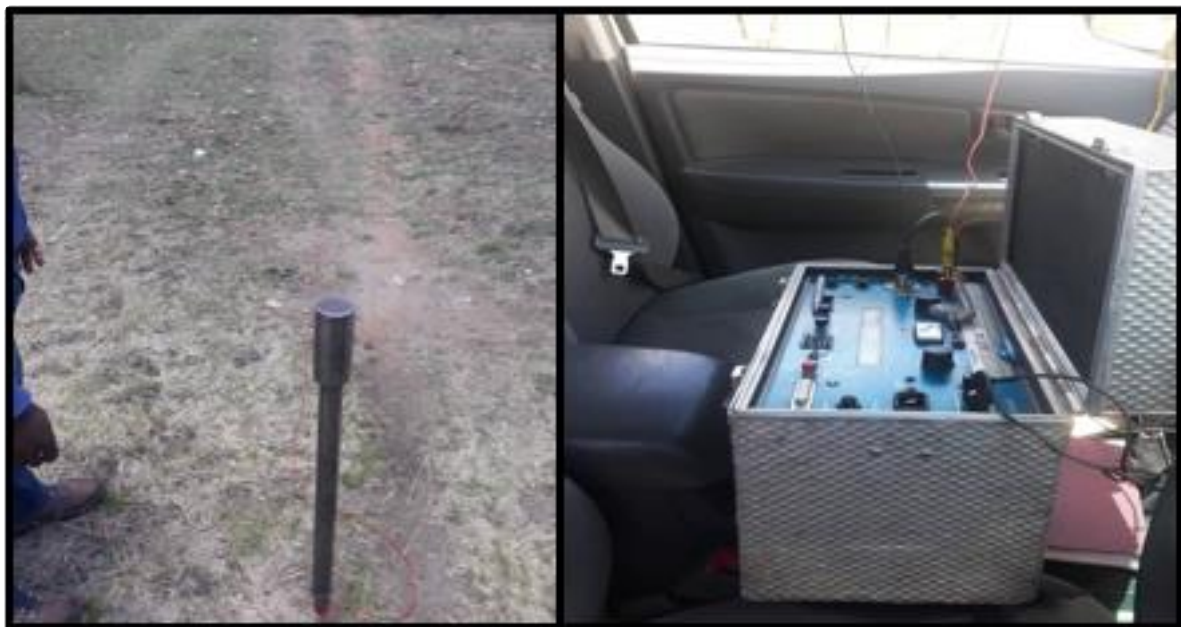
Fig 4.7. Field set up used for vertical electrical sounding on the experimental sites
