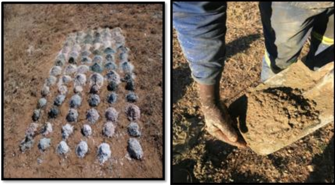
Fig 5.3. Sampling during air-rotary drilling
