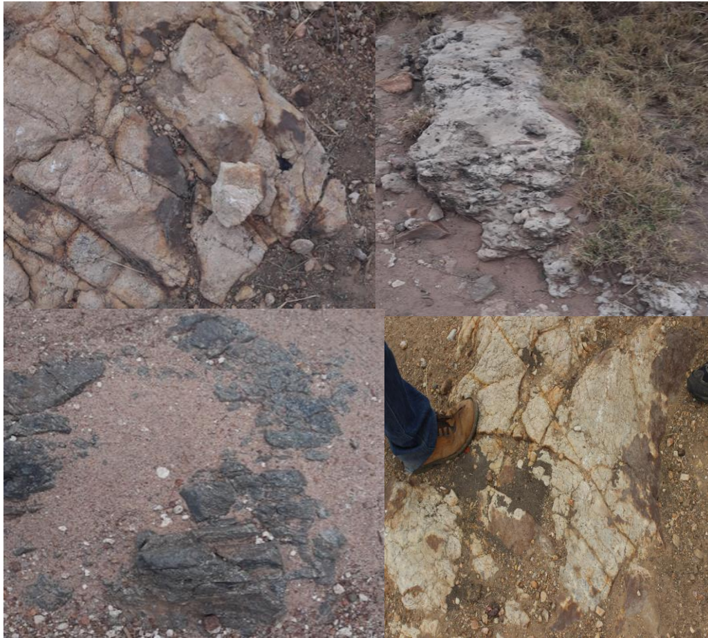
Figure 3. 4. Major geological features that control groundwater interaction in site three showing the fractured Hout river gneiss, intrusive dykes and a calcrete layer forming within the site.
