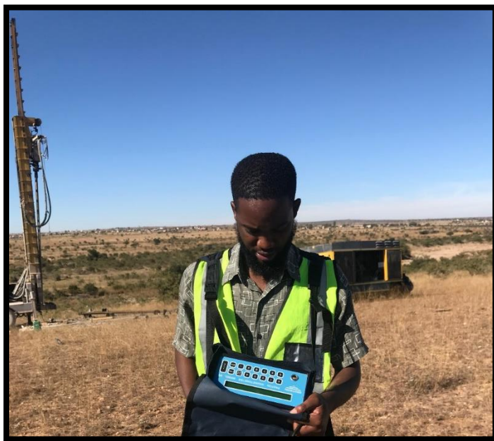
Figure 4.5. A G5 Proton Memory magnetometer used to conduct geophysical measurements.
