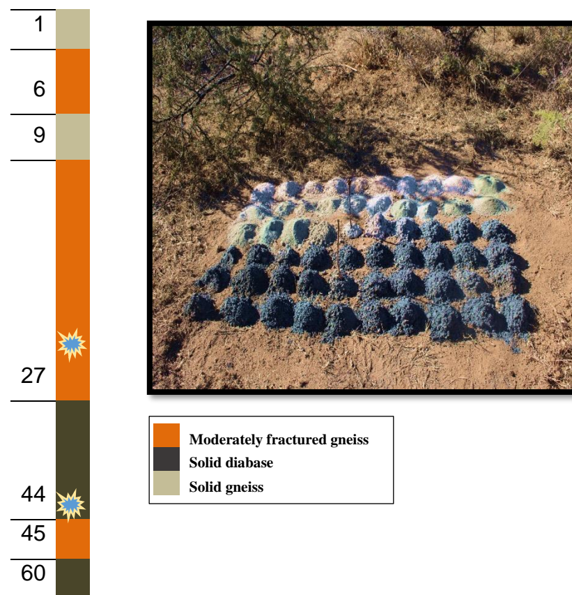
Fig 5.5. well profile and sample images for borehole HO4-3125
