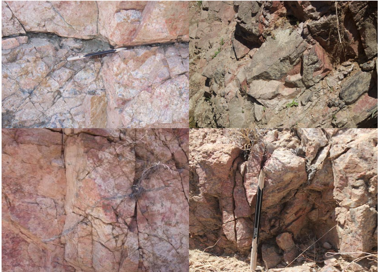
Figure 3.6. Photographic image of rock units showing the extent of fracturing within the Hout river gneiss at Site 4.
