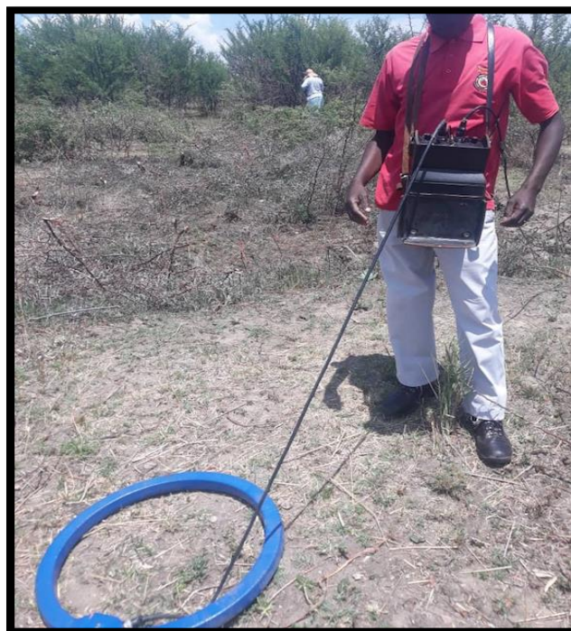
Fig 4.6. Conducting the electromagnetic method with the support of the Department of Water and Sanitation.
