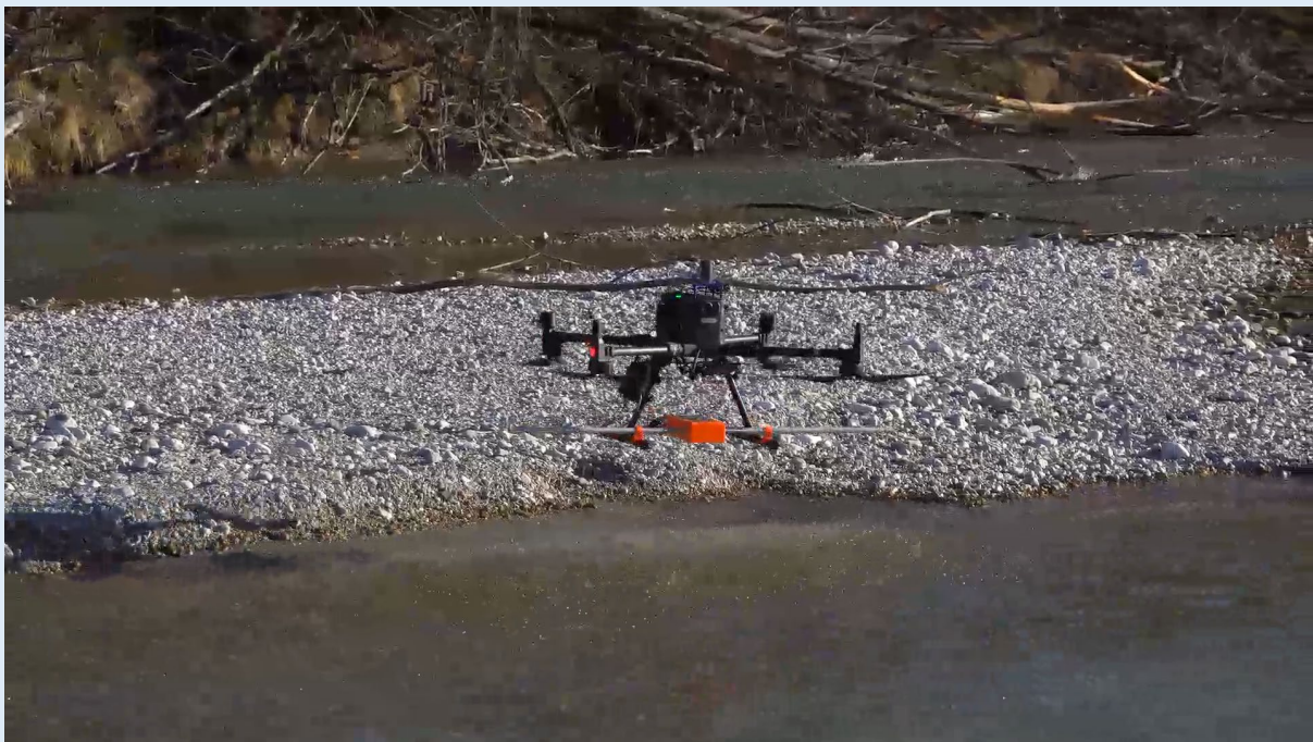
UAWOS water penetrating radar drone payload
