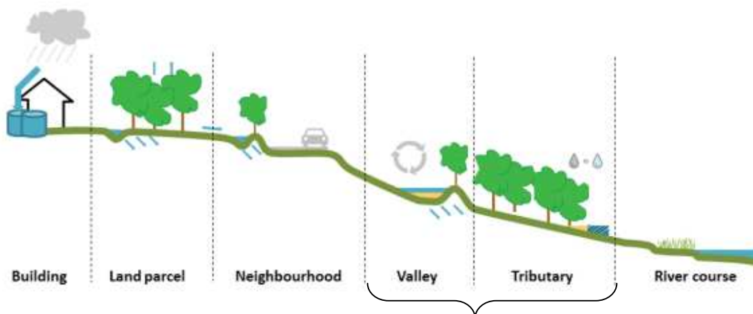
Figure 3. Longitudinal section of the suggested stormwater management train at different spatial scales Source (Report II)
